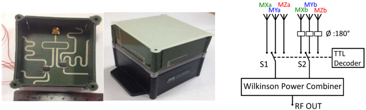
Figure 3-2: Fabricated antenna system on top of a commercial package (left), switching diagram (right).
